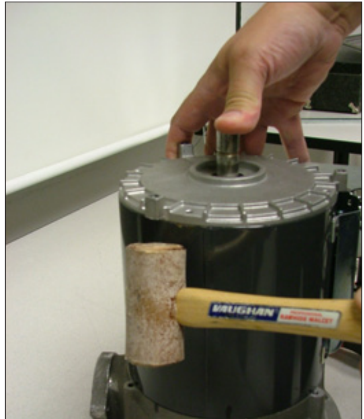
Figure 30. Marking and Removing Lower End Framer
