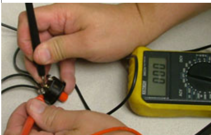
Figure 24. Testing Overload Protector
