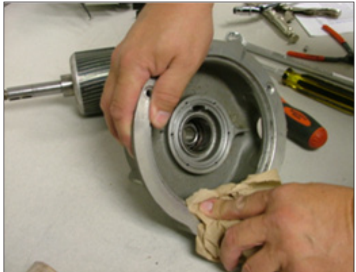
Figure 21. Cleaning Upper End Bell
